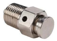
They are all spring loaded and made of resilient materials such as Brass or Stainless Steel. These nifty labor saving devices eliminate the need for a tower climber and allow you to purge your system at will, any time you desire. These poppers are ordered with specific "crack open" pressure levels that range from 1 psi to 200 psi. If your Nitrogen gets stinky, just purge it. Poppers are available with rain hats that keep contaminants out of the seals and the seal types are also selectable.
