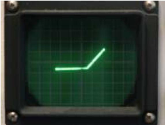
Resistive Junction, Leaky, Figure 4a
