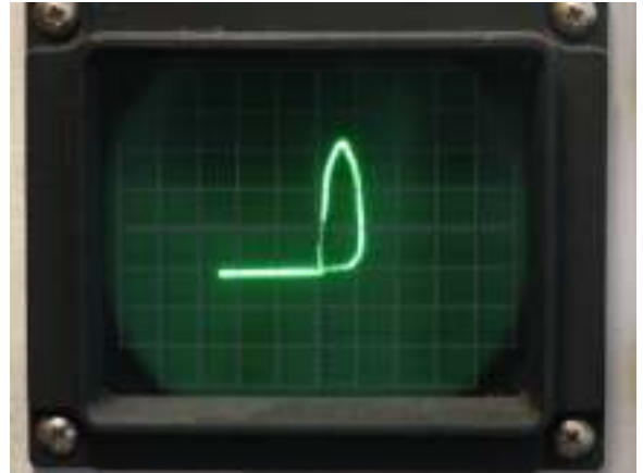
Capacitive Junction, Figure 4b
