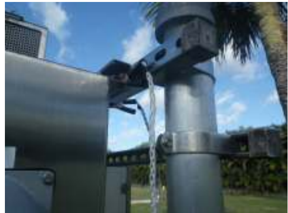
EXAMPLE OF CONNECTION FOR CONTINUITY TESTING
