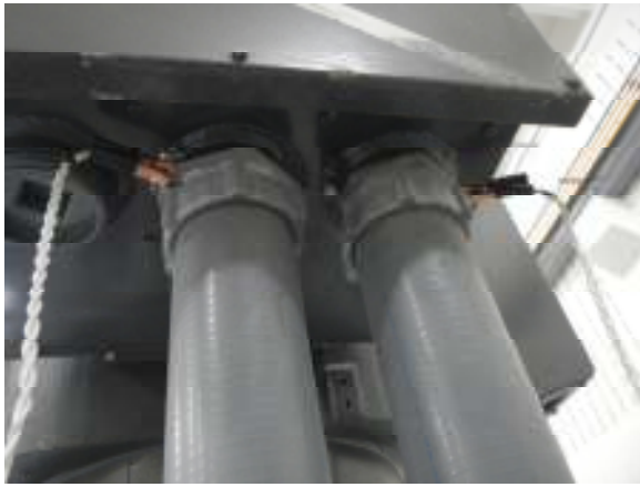
EXAMPLE OF TEST CONNECTION ON MEMBRANE PUMP
