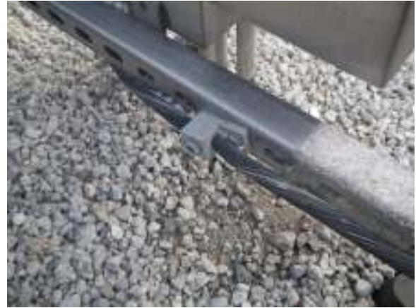
CORRODING SCREW SET TERMINAL
