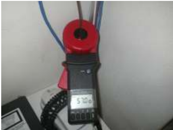
SINGLE END GROUND ROD IN TELEPHONE SHELF
