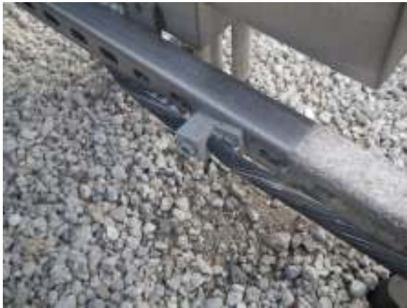
CORRODING SCREW SET TERMINAL
