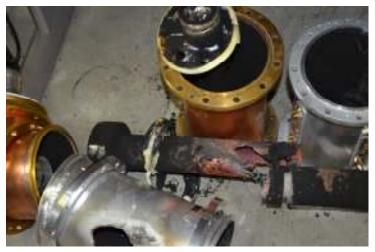
Having lost the coaxial switch, the in line tuner attached to the output of the final hybrid melted sufficiently to leave a pile of molten Aluminum on the floor and destroy the R.F. monitoring coax cables along with the switch operation cable that were attached to it.
