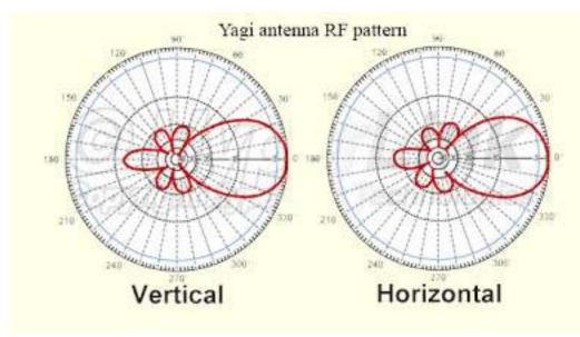
Lastly for our example the Yagi as it is abbreviated, has similar pattern abilities to the panels antenna but the rear radiation of the Yagi is higher and less controlled though the gain can vary from only a few dB to over 26dB in some cases. Notice how
